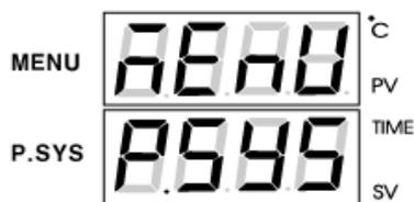
4. After P.SYS displayed, Press the "Mode" key continuously
